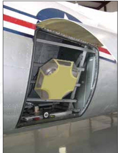
FIRST RF's UHF SAR antenna reduces volume relative to horn in this DC-3 aircraft.
