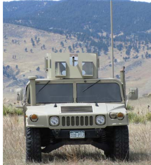
FRF-172 Spring Mount Antenna on HMMWV
