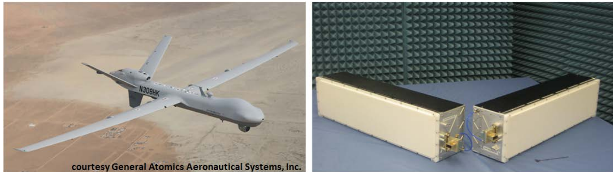
General Atomics Predator B equipped with FIRST RF X-band Active Electronically Steered Array (AESA)
